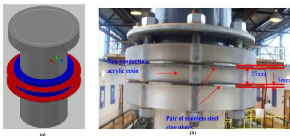
Figure 2. Conductance ring probes (a) impression of the calibration set-up with the conductance probe rings (in red), a water portion (in blue) and the non-conducting cylinder (in grey) [6] (b) the parallel conductance ring probe [4].
