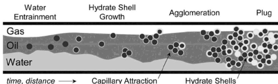
Fig. 1. Hydrates formation in pipelines [39].
