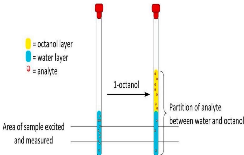
Fig. 2. Schematic representation of Analyte Partition between the water and 1-octanol Inter- Phase at Equilibrium [45].
