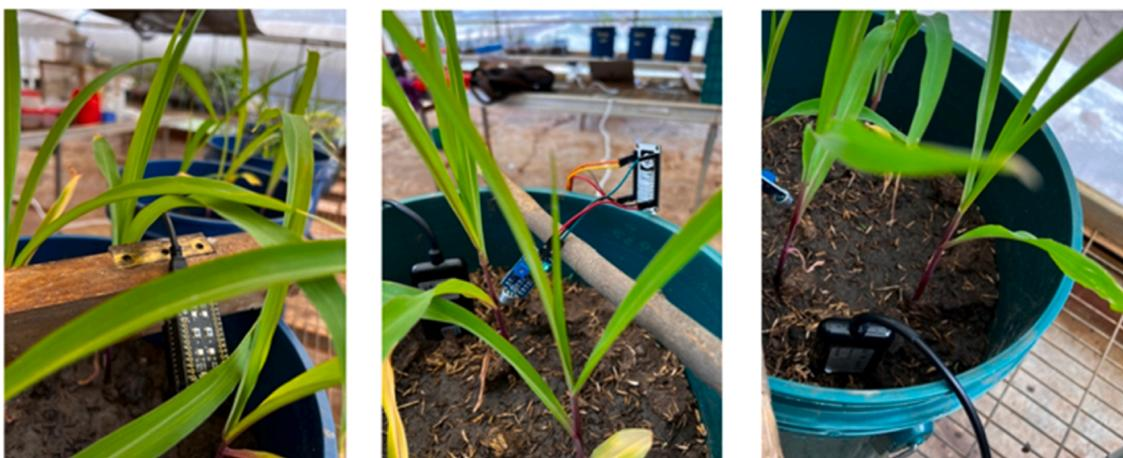
Fig. 4. VOC, Ultrasound and NPK sensors on planted maize crops.
