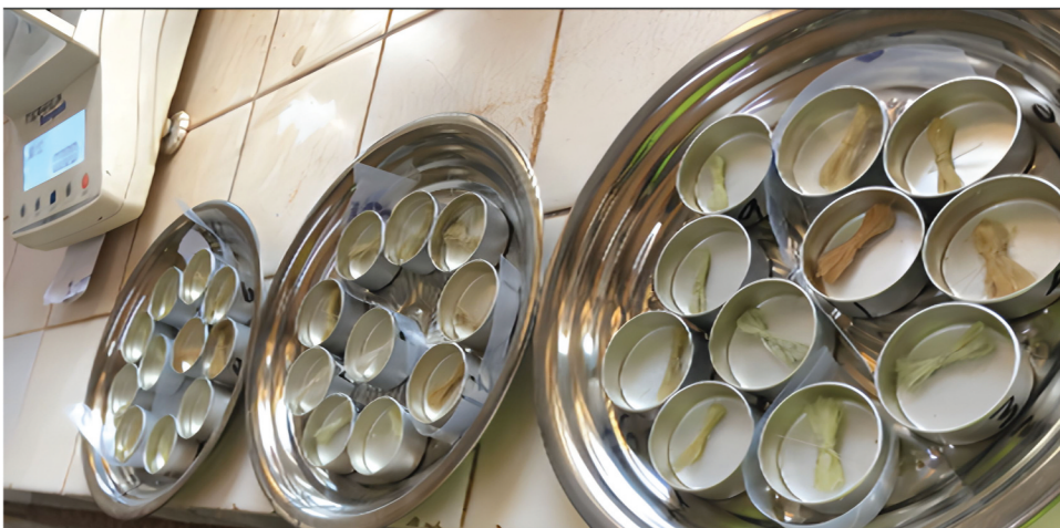
Figure 1. Water absorption tests for raw and different treated sisal fiber.
