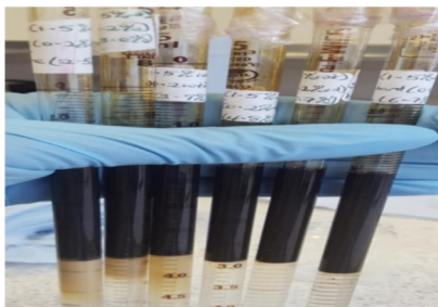
Figure 9. Phase separation of 3.0% of the OME in hard brine and crude oil at 80 °C.
