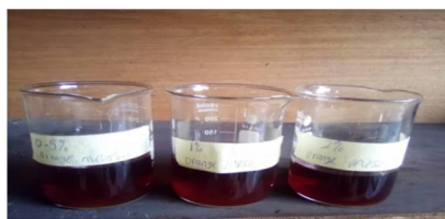
Figure 5. Compatibility test of OME in soft brine at 80 °C.
