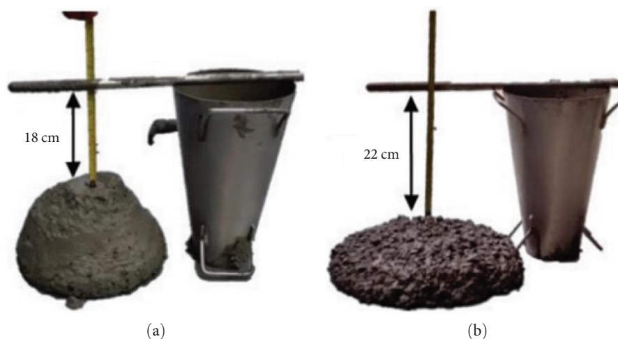
FIGURE 1: Slump test of concrete mixture (a) only by OPC and (b) OPC + alkali activated by natural pozzolana from Robayo-Salazar et al. [58].
