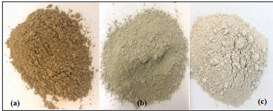
Fig. 1. The colour difference of used (a) blast furnace slag, (b) raw bentonite, and (c) active limestone. (For interpretation of the references to colour in this figure legend, the reader is referred to the Web version of this article.)
