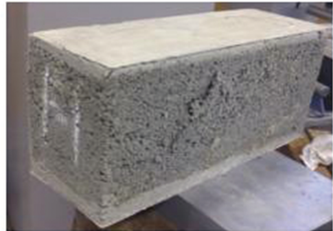
Sisal fiber reinforced concrete block
