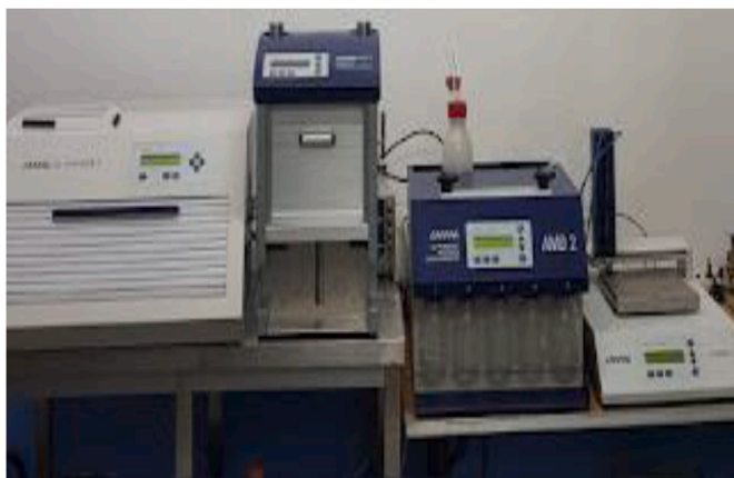
Fig. 4. CAMAG semi-automatic HPTLC system.
