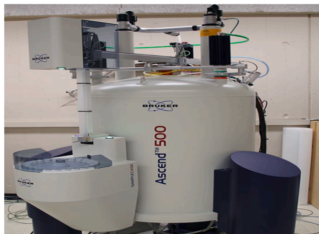
Fig. 3. Nuclear magnetic resonance spectrometer (Bruker Avance III, 500 MHz).
